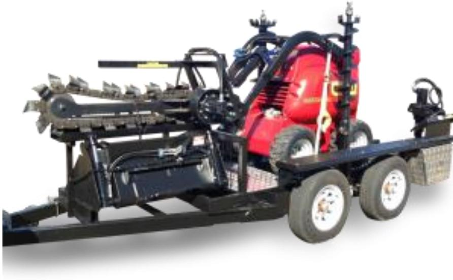
This trailer has some great features: Tilt deck ramps that make it easier and safer to load especially for novice users; over-ride brakes so will be suitable to tow behind most utes; tandem axle so there will be less weight on the tow vehicle
