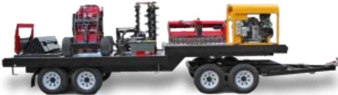
This trailer is designed for the contractor who needs to carry a lot of gear. The trailer has a 6m deck with a step of 200mm at 2.6m.
